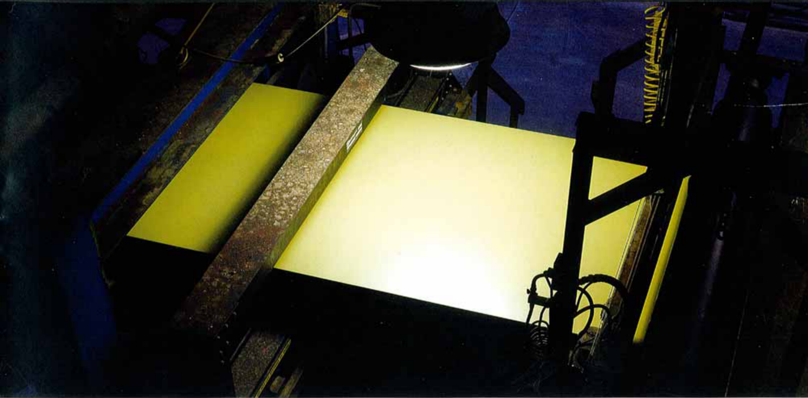
A painted strip passes under inspection lights where it is checked for defects.
