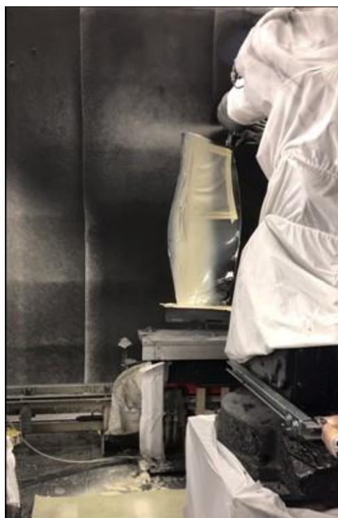
Figure 4: Conveyorized Robotic Paint Application
