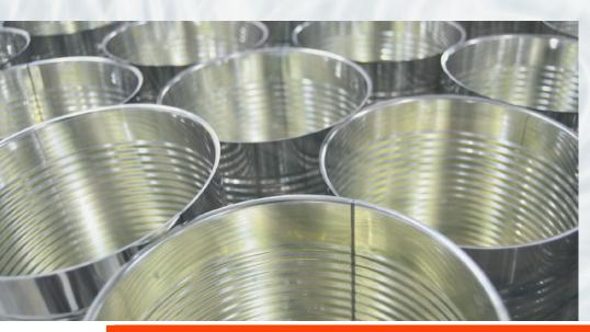
Saint Clair Systems works with a 3-pc. can manufacturer to reduce variation in their end liner operation. Controlling the material temperature stabilized the pressure at the nozzle and yielded some extraordinary results.
