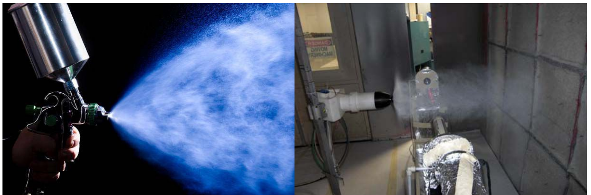
FIGURE 1. Gun 1 vs. bell 2 atomizers
