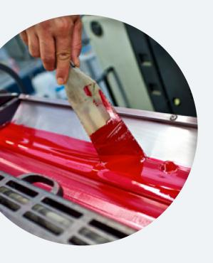
Inks are highly viscous under normal conditions, but will gradually become less viscous as force or stress is applied. Removing ink from the process eliminates the effects of shear. This ultimately ensures that you will not get an accurate process reading.
