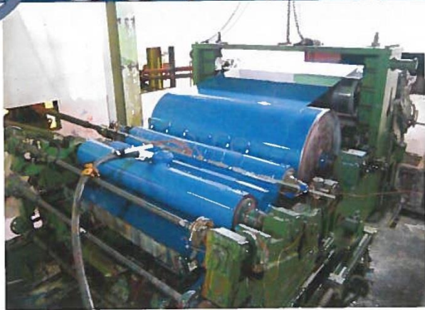
Figure 4: 3-Roll Reverse (Indirect) Nip Feed Configuration
