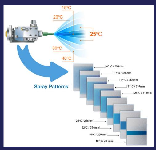
Here we can see how the spray pattern changes, with the width increasing proportional to the temperature. This phenomenon is caused by the change in viscosity. **So, when we talk about temperature, we are talking about viscosity.**
