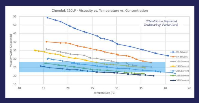
In the chart above, we see the viscosity-temperature curves for various dilutions of Parker Lord's Chemlok 220. Parker Lord's DS3105 data sheet recommends applying this coating at a viscosity of 22–28 seconds which indicates that you must dilute the material before spraying, (shaded in blue on the chart).
