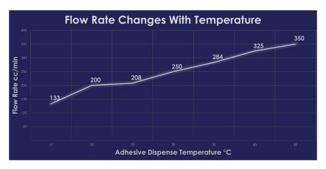
In the chart above, we see the flow rate-temperature curve for a 10% diluted Parker Lord's Chemlok 220. **Without constantly monitoring flow rate shifts, this process will see changes in spray pattern, coating thickness, and overall material consumption.** While this chart represents only 10% dilution, we saw the same relationship across a variety of dilutions from 0% to 50%.
