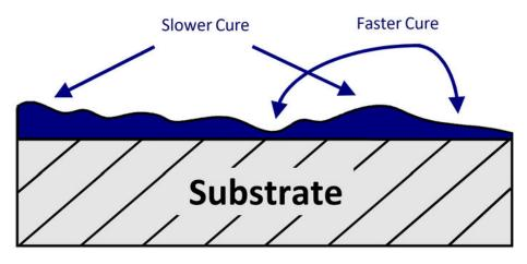
This uneven surface will have a negative impact on bond performance and can also promote the creation of blisters caused by solvent entrapment under the cured surface of the coating. Additionally, if the thinner film areas are at or above the minimum film specification, the thicker film areas represent excess coating applied which increases the coating cost.
