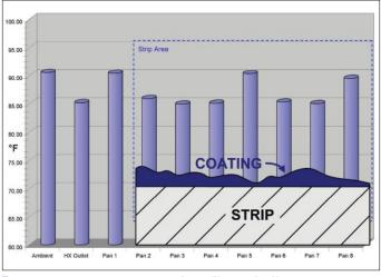
**FIGURE 10:** Uncorrected profile and effect on film build
