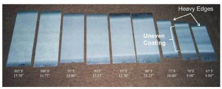
FIGURE 3: Effect of temperature on spray pattern
