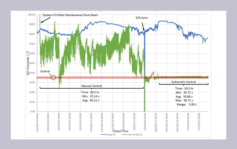
SUMMARY: Saint Clair Systems displaced a manual viscosity control process with automation. The automated viscosity control system generated a 97% reduction in viscosity variation, resulting in decreased material usage and increased throughput.
