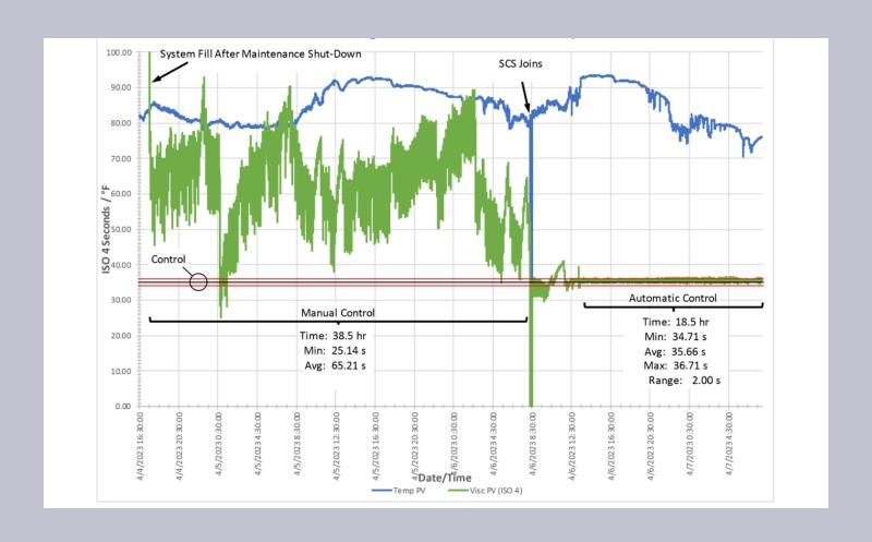
SUMMARY: Saint Clair Systems displaced a manual viscosity control process with automation. The automated viscosity control system generated a 97% reduction in viscosity variation, resulting in decreased material usage and increased throughput.
