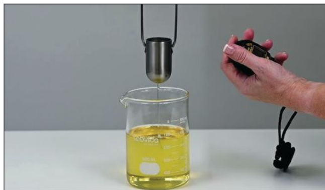
FIGURE 13. Manual viscosity measurement.
